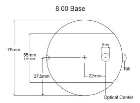
The optical center of the 8.00 base is in an 8mm diameter circle, 22mm from the geometric center, along a line connecting the geometric center and the center of the tab. The 6.00 base is NOT decentered.
